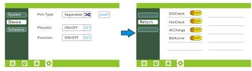
The function options in this navigation column are turned on and off for debugging. Please turn them off carefully, otherwise it may cause the machine to run abnormally or be damaged. Click "return" to return to the previous menu.
