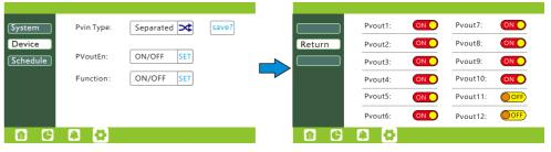
The user can choose to turn off certain channels of output, as above, ON means that the corresponding output is turned on, and OFF means that the corresponding output is turned off.
